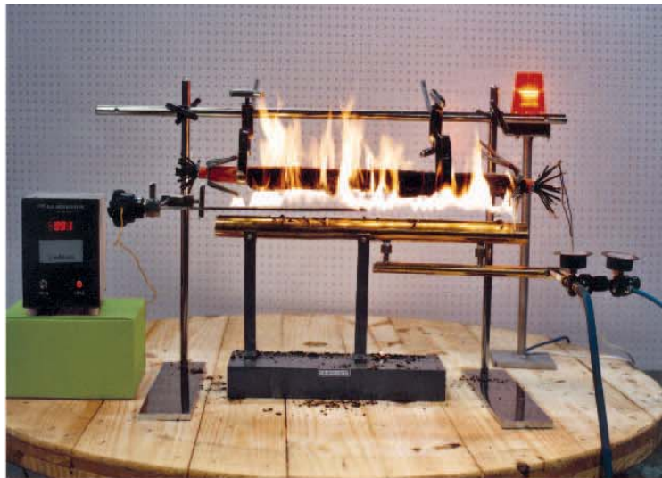
3 Hours fire survival test as per IEC-331
